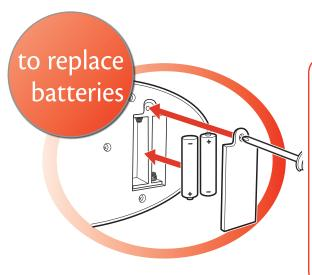
Use a Phillips/cross head screwdriver (not included) to loosen screw in battery compartment door (screw remains attached to door). Remove door. Remove old batteries. Insert 2 "AA" or R6 size batteries. Alkaline batteries recommended. Replace door and tighten screw.
